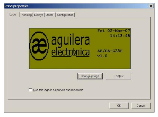
It is possible to include any image in BMP format with a size of 144 \* 56 pixels in 2 colours.
