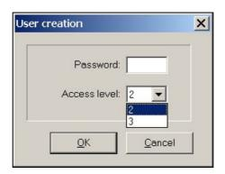
Only the access levels 2 and 3 can be established, in accordance with the EN 54-2 standard.
